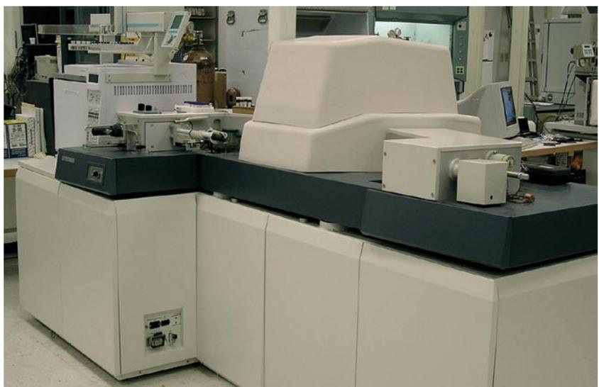
*The Autospec Ultima HRGCMS by Micromass can quantitate Polychlorinated Biphenyls in a variety of matrices to part-per-trillion (ppt) and part-per-quadrillion (ppq) levels.*
