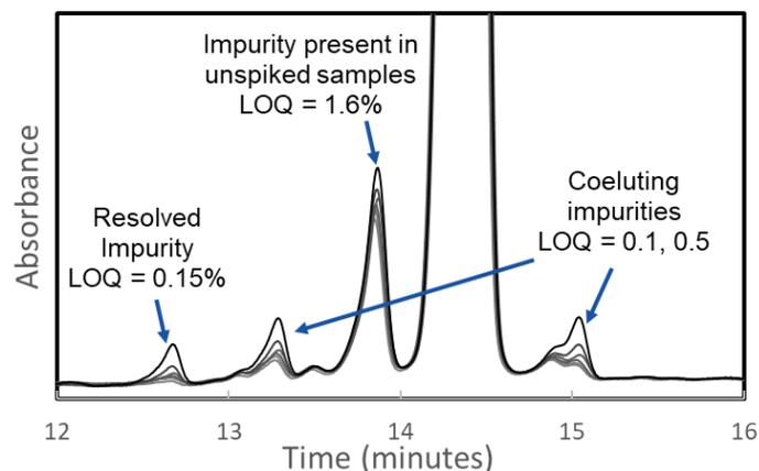
**Figure 4.** Validation experiments require careful design and selection of impurities when determining LOQ.
