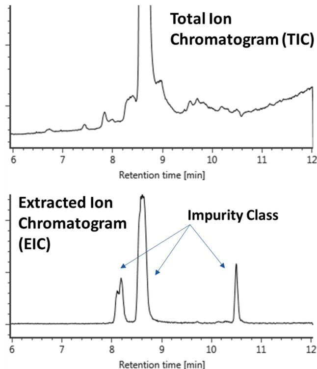
**Figure 3.** LCMS methods identify impurity peaks and can quantitate impurities coeluting with the main peak.
