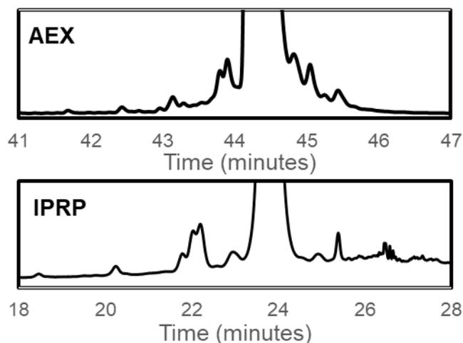
**Figure 2.** Orthogonal methods resolve more impurities collectively providing better manufacturing control.
