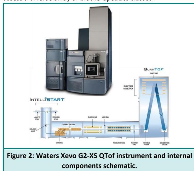
Figure 2: Waters Xevo G2-XS QToF instrument and internal components schematic.
