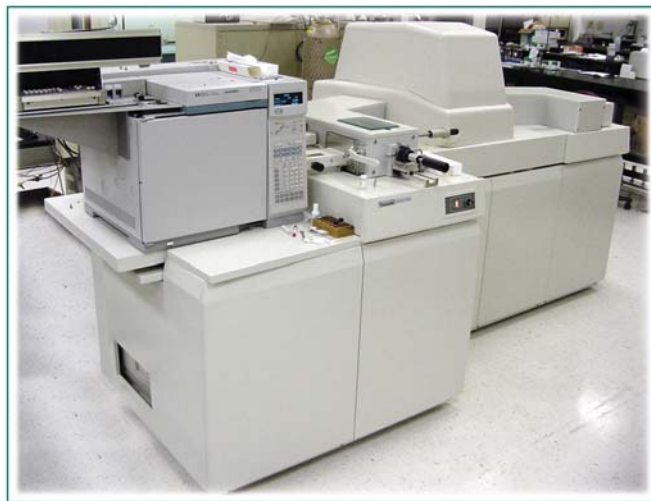
The Autospec Ultima HRGCMS by Micromass can quantitate Polybrominated Diphenyl Ethers in a variety of matrices to part-per-trillion (ppt) levels.
