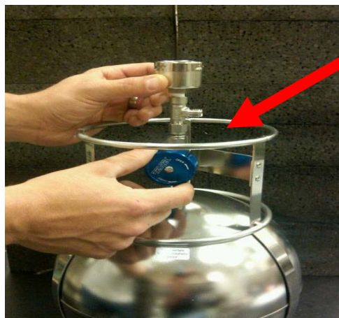
Sample Connection Point
