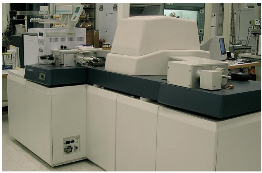
The Autospec Ultima HRGCMS by Micromass can quantitate Polychlorinated Biphenyls in a variety of matrices to part-per-trillion (ppt) and part-per-quadrillion (ppq) levels.
