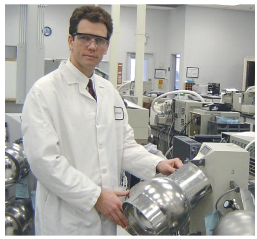
Summa canisters are the media of choice for vapor intrusion.
